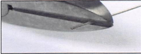
1A. Cut tube within 1/2" from exposed open end with wire cutter.
