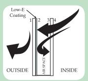
In cold weather conditions, the coating on the #2 surface reduces room heat (or infrared energy) from transferring across the airspace toward the outside. By adding a second Low-E coating to the #4 surface the thermal insulation is improved.
